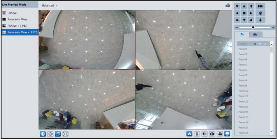
**4PTZ view mode** (you need to switch the stream mode in the fisheye parameter interface)
