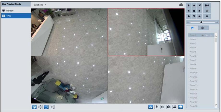
In panoramic + 3PTZ view mode or fisheye + 3PTZ view mode or 4PTZ view mode, select a PTZ window and view the image from every direction by controlling PTZ panel.
