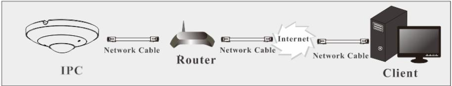
① Make sure the camera is connected via LAN and then log in the camera via LAN and go to Config→Network→Port menu to set the port number.
